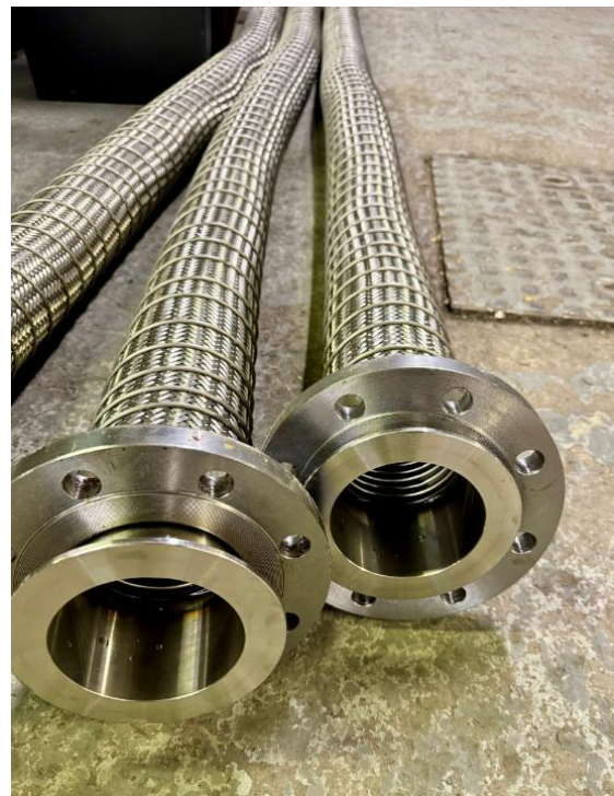
Flat Guard (left) and Procoil flexible hose protection
