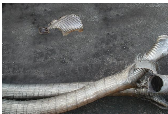
A burst flexible steam hose due to poor customer installation
