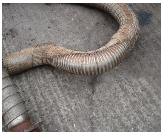
Very badly damaged protective braid and steam hose deformed
