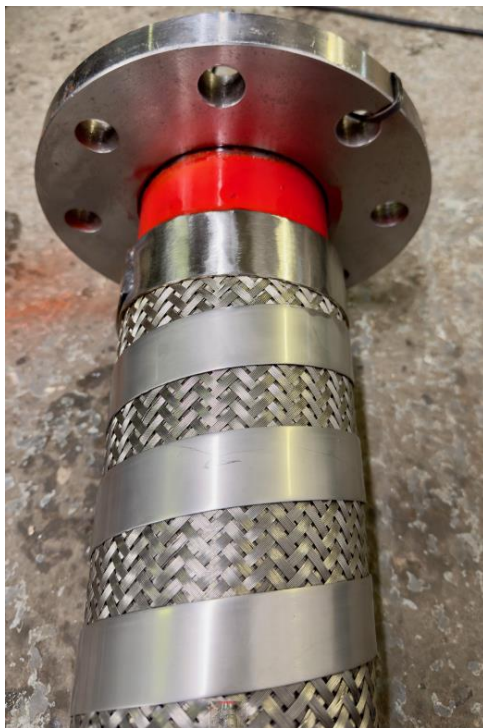
Flat Guard (left) and Procoil flexible hose protection
