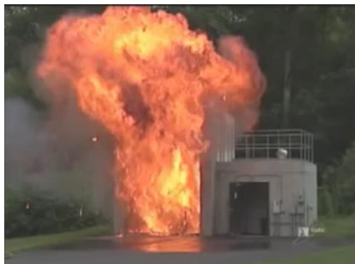
Image (Right) - Dust test explosion at FM Global's Research Campus, Rhode Island
