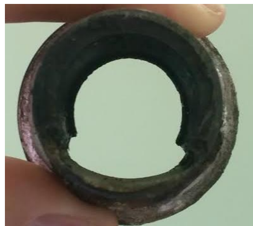
Figure 29 - Oxygen Pitting Corrosion Attack External View
