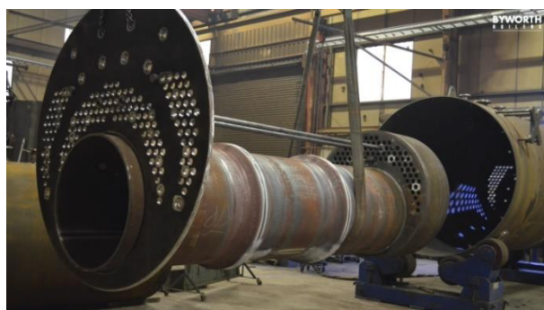
Figure 4 - Cut away image of standard shell boilers and a boiler under construction
