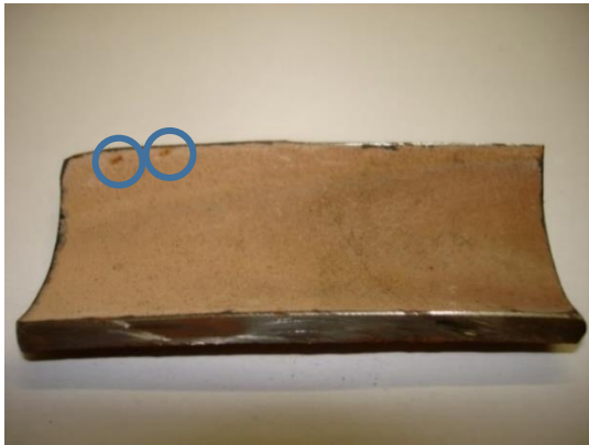
Figure 5 - Scaling of the internal surfaces of a coil boiler with corrosion underneath the scale as highlighted.
