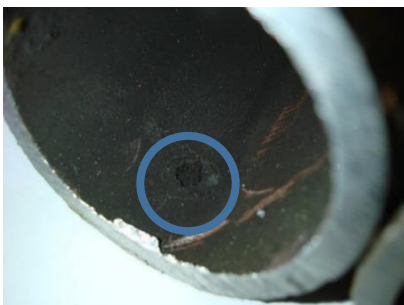
Figure 10 - Historic corrosion pit covered by a new magnetite layer after an acid clean
