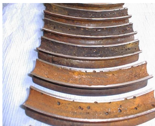
Figure 28 – Coil Boiler Tubes Cut Away View showing Oxygen Pitting Corrosion Attack
