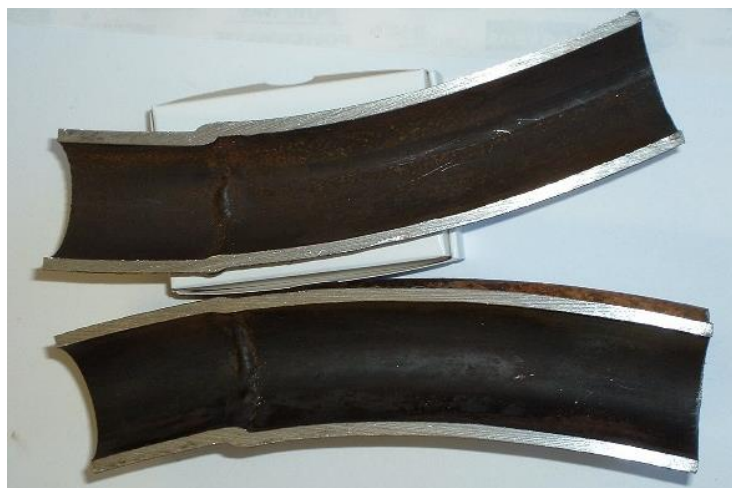
Figure 48 - A well-treated steam generator coil-internal cut away view showing well-formed magnetite layer internally
