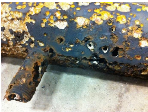
Figure 29 - Oxygen Pitting Corrosion Attack External View
