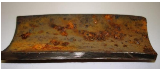
Figure 27 – Coil Boiler General Corrosion Attack
