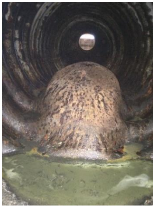
Figure 8 - Boiler Furnace Deformation. This could have been a complete catastrophe
