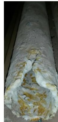
Figure 6 - Scaling of the external surface of a tube in a shell boiler
