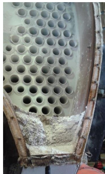
Figure 14 – Deposition caused by a leaking boiler tube
